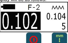
6.6.2.6 Use buttons and for setting adequate average measurements to the rated value of the thickness of the covering.
